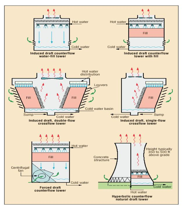
Figure 7.2 Cooling Tower Types
