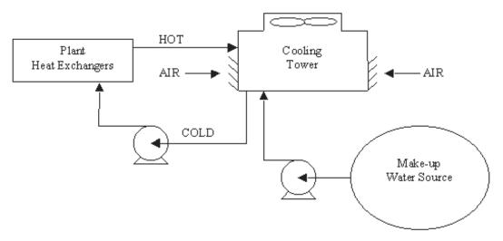
Figure 7.1 Cooling Water System
